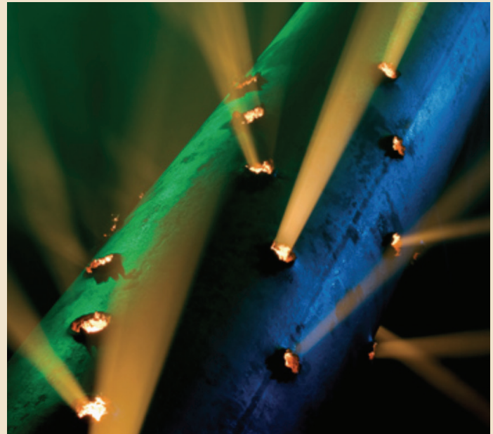
^ High shot density casing gun after perforating.
