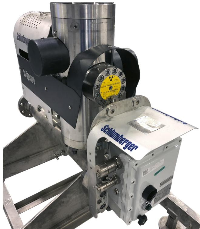
*AquaWatcher Surface water salinity sensor integrated with the Vx Spectra surface multiphase flowmeter.*
