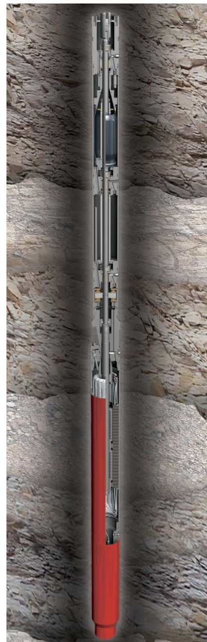
Figure 1. Schematic of the ProMotor unit illustrates how integrated, factory-filled motor, protector and gauge are combined with plug-and-play power connector to eliminate weather and skill-dependent field assembly procedures. (All graphics courtesy of Schlumberger)
