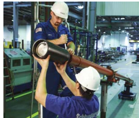
Figure 4. Factory crew installs compensating shipping cap after topping off the unit with clean dielectric oil.
