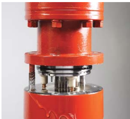
Figure 2. Upper MaxJoint flange connection features sealed shaft and automatic oil communication valve, while oil-filled lower unit remains filled with pure oil and eliminates trapped air when the two are mated.
