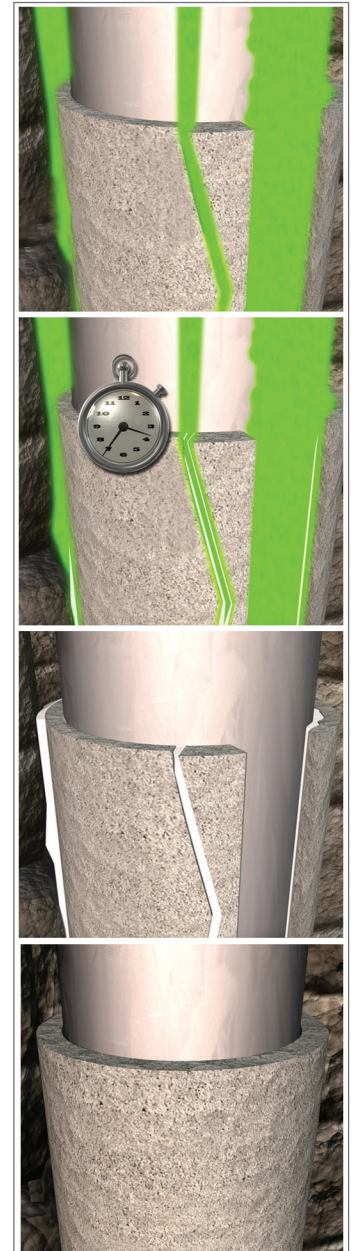
Hydrocarbon flow (shown in green) activates FUTUR active set cement whenever the integrity of the cement sheath is compromised, efficiently sealing the leak path and reestablishing well integrity.
