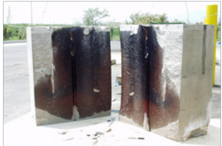
Block broken open to reveal hydraulic fracture surface; from experiment by Casas et al.
