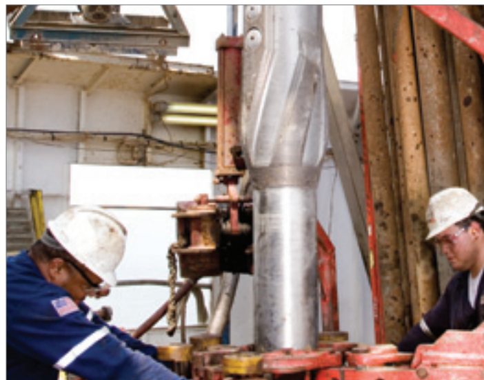
The StethoScope 825 service uses an 8¼-in collar with a 12-in integral blade stabilizer for 12¼-in boreholes. An optional collar with a 10⅝-in stabilizer is available for 10⅝-in boreholes.
