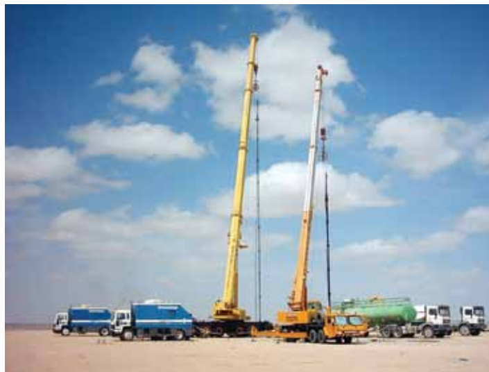
Deployed on standard wireline equipment, the transmitter and receiver tools of the DeepLook-EM crosswell electromagnetic system directly measure the interwell resistivity.
