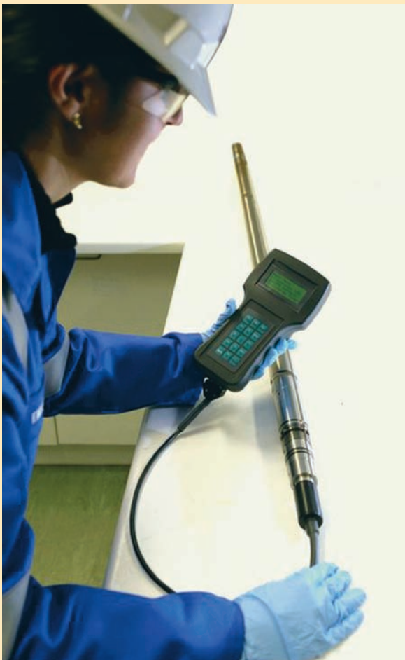
A technician uses the hand-held programmer to pre-set the actuation time of the Compact Production Sampler before running it into the hole
