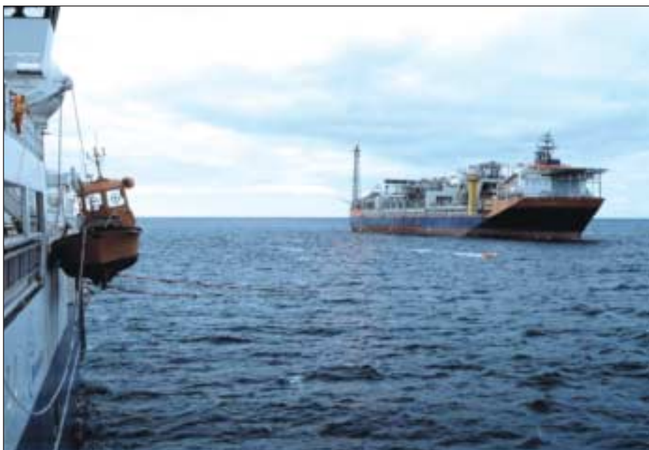
▲ Acquiring seismic data near the Norne FPSO. The Geco Topaz towed seismic streamers within 40 m [131 ft] of the Norne FPSO. The outermost streamer is trailing the orange buoy on the right of the photograph.
