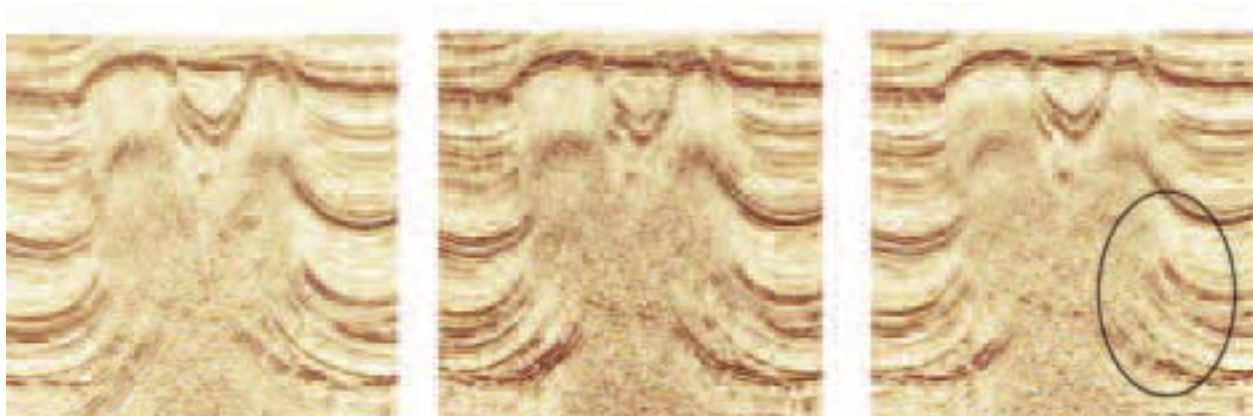
Figure 4 Kirchhoff pre-stack time migration. Left picture shows the E-W survey only, middle picture shows the N-S survey only, right picture shows both surveys combined. Note the smearing of events on the combined data set.
