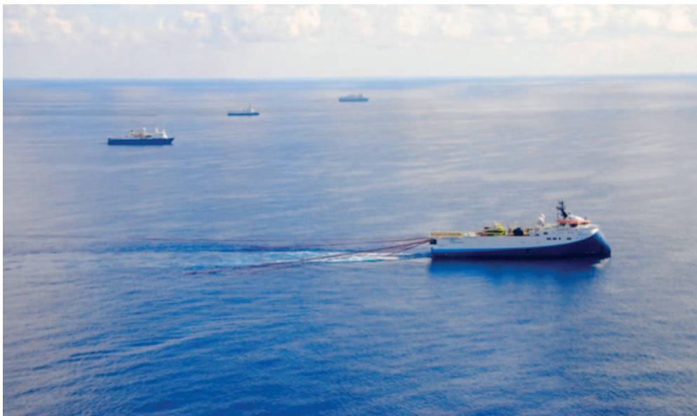
Modern wide-azimuth acquisition typically utilizes four or more vessels. (Images courtesy of WesternGeco)
