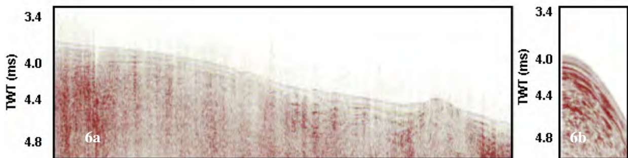
Figure 6 Difference plots showing multiples attenuated through use of 3DGSMP for (a) Crossline stack and (b) CMP gather
