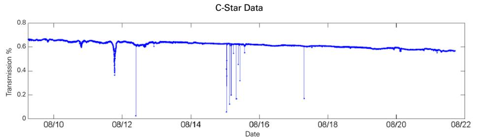
*The TURBIDITY and METOC services instruments deployed on the USVs show evidence of suspended sediment plumes, rendered as increased backscatter and decreased transmission.*
