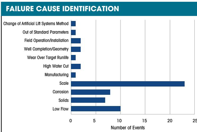
**FIGURE 1.** This chart shows the failure distribution for the sample wells. Post-failure analysis identified failure cause for 58 events for the sample wells. As scale failures were seen in the same well, this was a well-specific problem rather than a field trend. (Source: Schlumberger)
