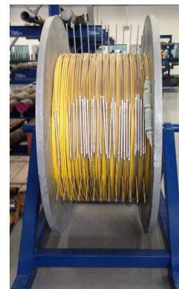
*The WellWatcher Flux system includes arrays of miniaturized, hermetically sealed digital temperature sensors connected to a single electric cable.*
