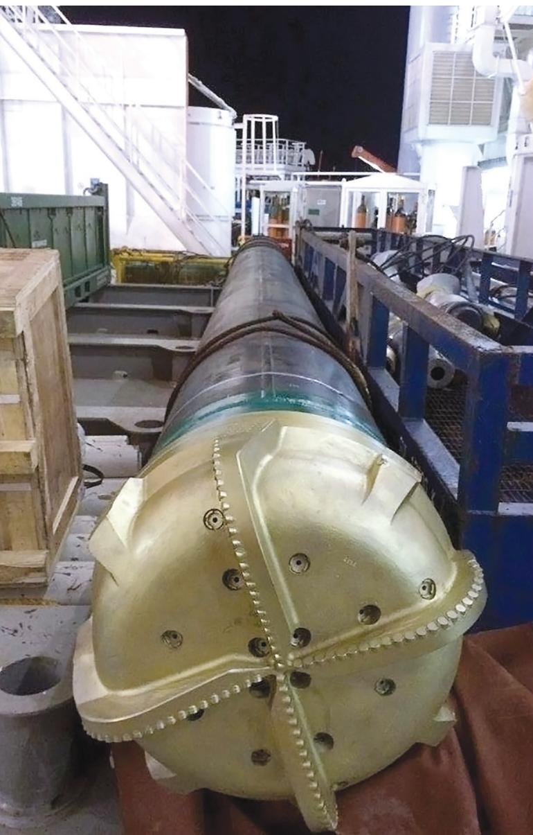
The first 34-in. PDC drillbit from the Schlumberger Direct XCD drillable alloy casing bit portfolio was specially designed for drilling two challenging shallow-water exploration wells in the Gulf of Mexico. (Source: Schlumberger)
