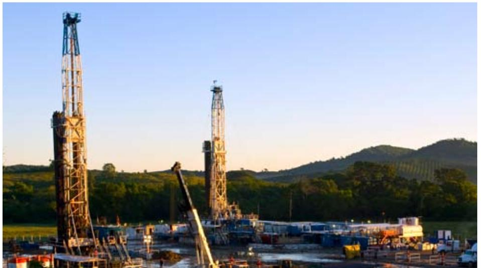
*Two Factory Drilling operations on the same pad in Mexico. Simultaneous operations (drilling, completion, production) lead to increased efficiency, lower environmental impact, and fewer access roads.*
