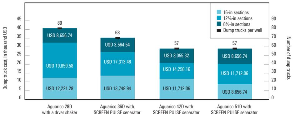
Implementing the SCREEN PULSE separator helped Consorcio Shushufindi reduce the total mud on cuttings and cut down on the costs associated with waste disposal.
