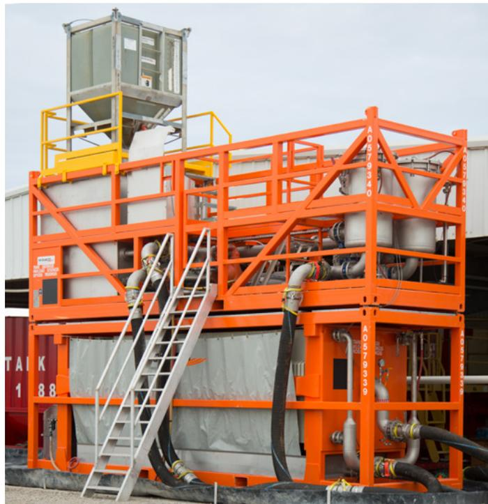
*The Torrential unit filtered 4,600 bbl of clear-brine completion fluid in 4 hours—a 47% improvement over standard filtration equipment.*
