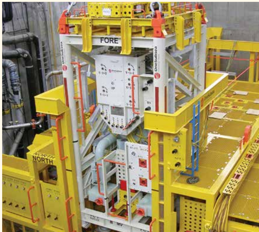
The OneSubsea single-phase pump systems for the Stones wells consist of a fully encapsulated pump and motor, designed for 10,000-ft (3,000-m) water depth and internal pressure up to 15,000 psi. (Courtesy of Schlumberger)
