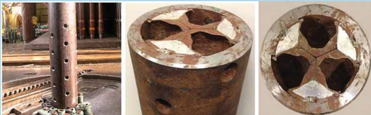
Examination of the spent 6 5/8-in. perforating gun incorporating INsidr perforating shock and debris reduction technology shows that the shaped charge cases do not break but remain in one piece, resulting in only negligible debris out of the gun. (Courtesy of Schlumberger)
