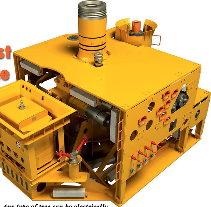
**Any type of tree can be electrically actuated regardless of configuration, illustrated by the OneSubsea horizontal tree, including electrical actuators and downhole safety valve interface (illustration: Schlumberger)**
