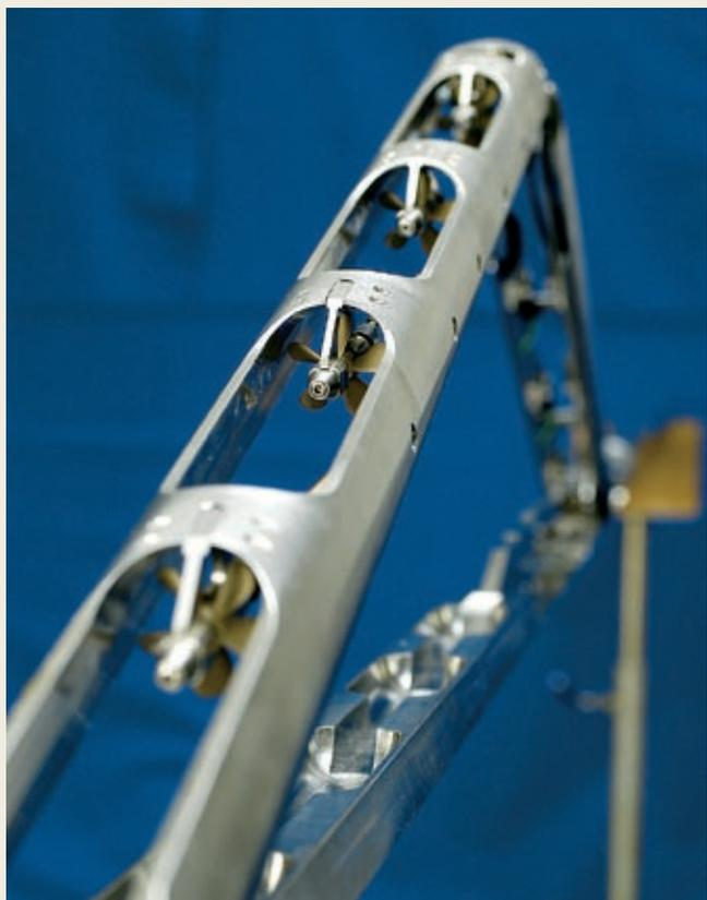
**Fig. 2.** Miniature spinners of this tool measure velocity at five different points across the wellbore's vertical axis, enabling calculation of a multiphase velocity profile.
