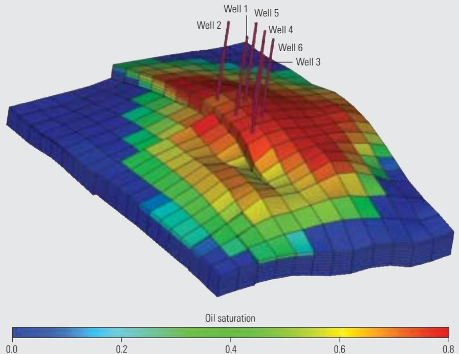
^ Reservoir model of the synthetic Charon field. This ECLIPSE reservoir model provided input for obtaining production predictions, using a large number of simulations with geostatistically derived porosity and permeability values.
