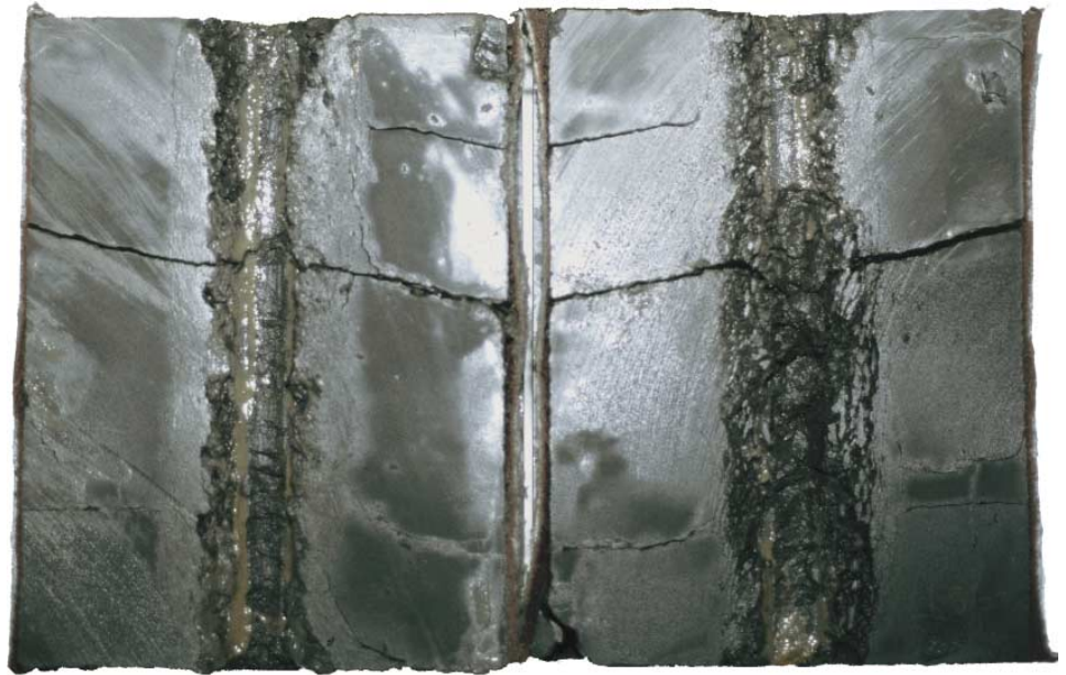
□ Shale instability. In this example, Pierre shale has been exposed to a mud comprising fresh water and bentonite gel. Because this fluid contains no inhibitors, water has entered the shale causing it to swell and weakening the formation. Continuous flow of mud has eroded the borehole leaving an enlarged hole that would be hard to log and complete. This simulation was carried out using the small wellbore simulator at Schlumberger Cambridge Research, Cambridge, England.
