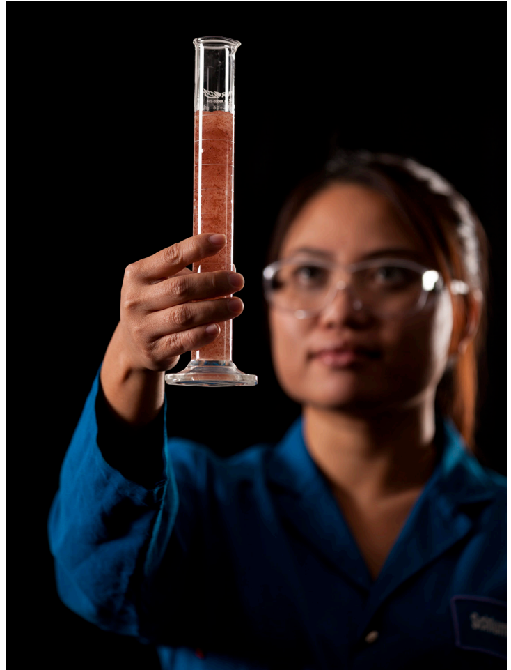
ClearPAC HT fluid suspended the ceramic proppant for gravel-packing at low rates, which was critical to avoid fracturing the formation.
