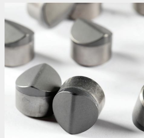
Figure 2. The new Axe ridged diamond element features a unique ridge-shaped geometry that combines the shearing action of a conventional PDC cutter with the crushing action of a tungsten carbide insert cutter. (Image courtesy of Schlumberger)
