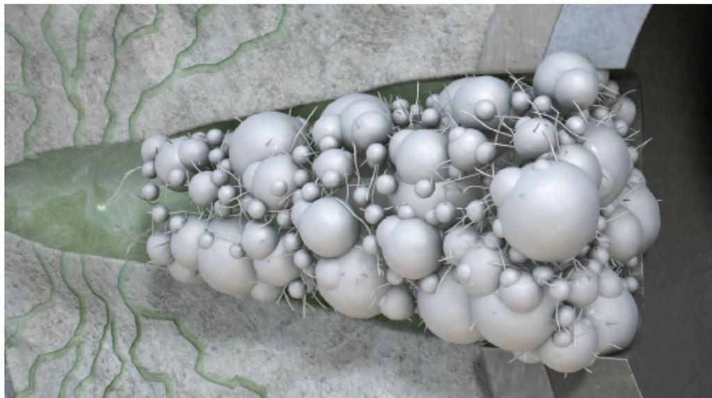
**The OpenPath Sequence diversion stimulation service sequentially plugs perforations in the near-wellbore to maximise wellbore coverage, resulting in greater production and recovery when compared with conventional methods. (Image: Schlumberger)**
