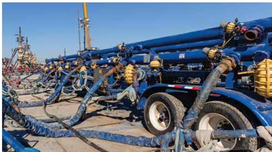
Yellow actuators on the valves of this missile manifold are about the only outward sign of the unit's automated capability. Without humans having to open or close these valves, a high-pressure risk has been removed and valuable time can be recaptured. *Source: Schlumberger.*
