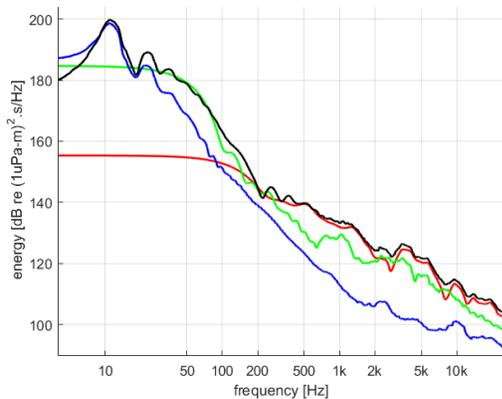
Figure 8: Decomposed amplitude spectrum of the new air-gun
