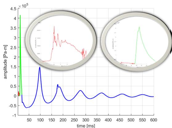
Figure 5: Measured signature of a standard 155 cu. in. air-gun, with close-up of the precursor (red) and main peak (green).
