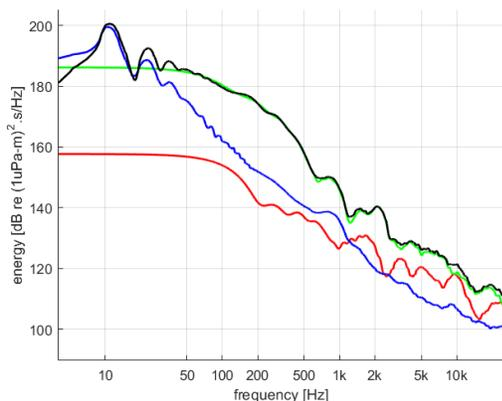
Figure 7: Decomposed amplitude spectrum of Figure 5 showing the contributions of the precursor (red), main peak (green) and free bubble (blue). The spectrum of the full signature is shown in black. The curves were generated by zero-padding the signature components, performing an FFT, and applying a one-third octave smoother.
