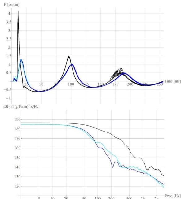
Figure 2: Signature of the new air-gun (configured for its most restrictive bandwidth and 150 cu. in.) as predicted by CFD (cyan) and as measured over 10 shots (blue); and measured signature of a standard air-gun (black) over 10 shots. Upper panel: time domain. Lower panel: frequency domain calculated over main peak.
