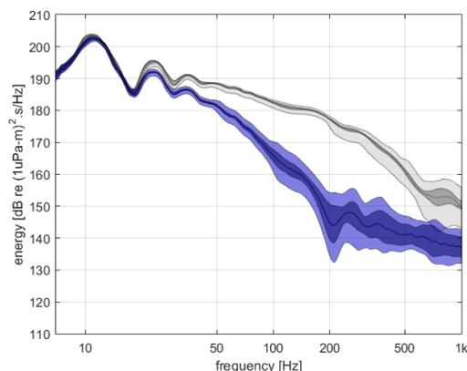
Figure 9: Expected range bands from shot variation for a standard air-gun (dark gray) and the new air-gun (dark blue); from manufacturing tolerances for a standard air-gun (light gray); and from the combination of manufacturing tolerances and long-term wear for the new air-gun (light blue).
