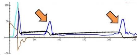
Figure 3: Measurements from sensors positioned inside an instrumented standard air-gun: Hall-effect shuttle-motion sensor (blue), fire-chamber pressure (black), and solenoid current (brown). Two secondary shuttle strokes (arrows) can be seen.
