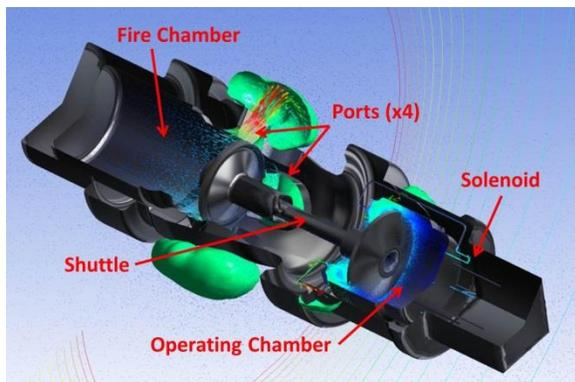
Figure 1: Internal components of an air-gun. The fire chamber is sealed with the shuttle in its left-most position.
