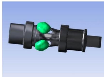
Figure 4: CFD simulation showing the precursor bubble immediately before the main release of air through the ports. At this stage the shuttle has just reached the beginning of the ports.
