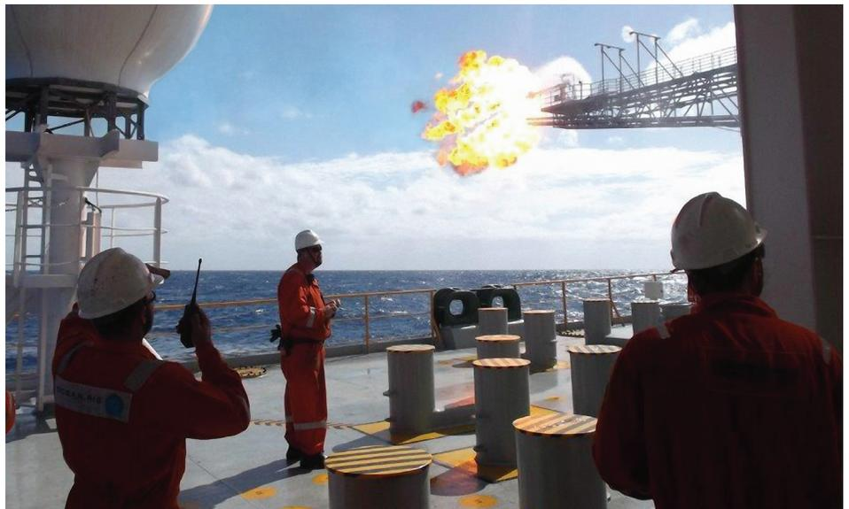
*Fallout-free, smokeless combustion of well effluent produced during well testing.*
