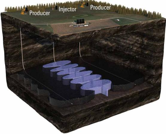
*The ResFlood system helps equalize the injection profile by restricting flow into high-permeability zones and encouraging injection into less permeable zones, improving sweep efficiency and recovery factor.*
