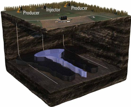
*Heterogeneous permeability and frictional pressure losses can lead to variable injectivity along long laterals.*
