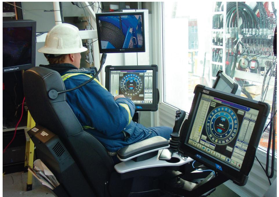
*With multiple screens and touch and joystick controls, the PRECISE system enables full control of drilling functions from a single source.*
