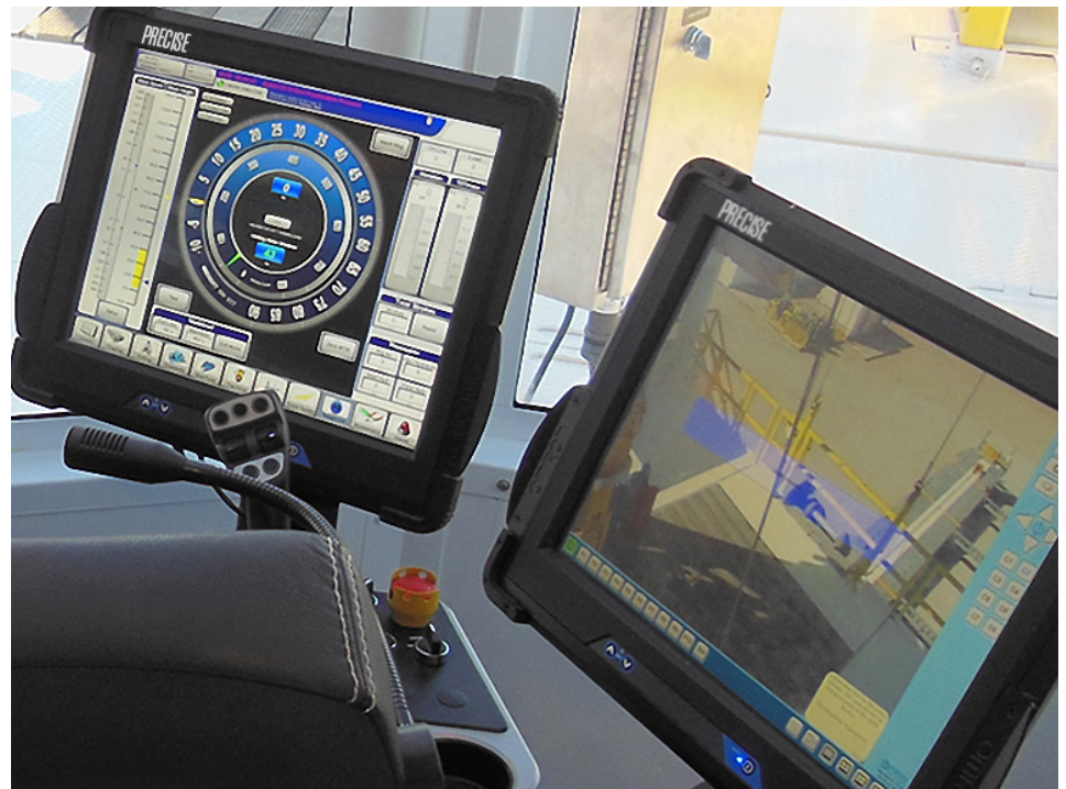
The SOFT TORQUE software plugin integrates seamlessly into AC VFD systems to mitigate stick-slip while rotary drilling.
