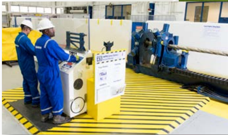
Crane bay breakout machine.
