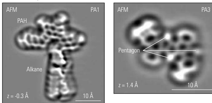
Figure 4. Asphaltenes. Atomic force microscopy (AFM) images of petroleum asphaltene molecules show polycyclic aromatic hydrocarbons (PAH) composed of fused six-membered aromatic rings and some alkane substituents. The pentagons are five-membered rings with some double bonds. These images support the molecular representation in the Yen-Mullins model. (Images used with permission, courtesy of IBM Research, Zurich, Switzerland. <http://dx.doi.org/10.1021/jacs.5b04056>.)
