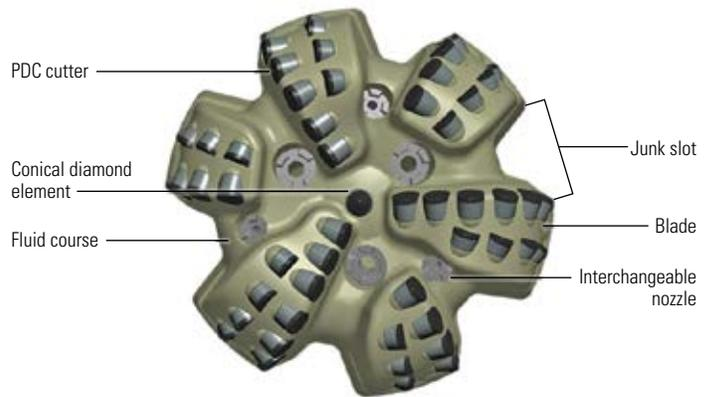
Figure 2. Face of a polycrystalline diamond compact (PDC) bit. The most prominent features of this bit are its blades and PDC cutters. Nozzles direct the drilling fluid downward to help break up the rock. Junk slots and fluid courses provide flow paths away from the bit face to aid in removal of cuttings.
