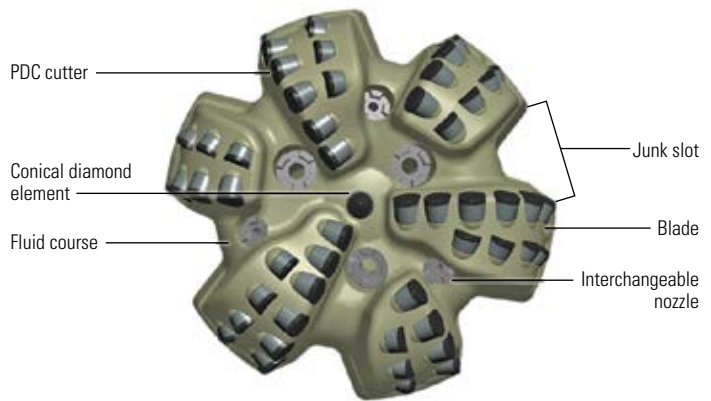
Figure 2. Face of a polycrystalline diamond compact (PDC) bit. The most prominent features of this bit are its blades and PDC cutters. Nozzles direct the drilling fluid downward to help break up the rock. Junk slots and fluid courses provide flow paths away from the bit face to aid in removal of cuttings.
