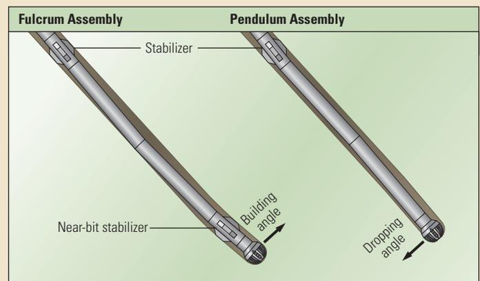
^ Using the BHA to change angle. Bending of the pipe above a bit influences borehole deviation. Through strategic placement of drill collars and stabilizers, the directional driller can increase or decrease flexibility and bowing of the BHA to build or drop angle.
