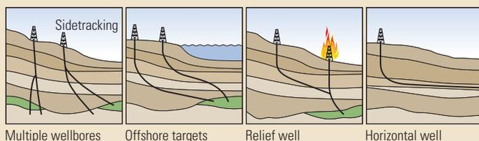
^ Directional drilling applications. Reservoirs that are not readily accessible from available surface locations can be exploited through directional drilling.
