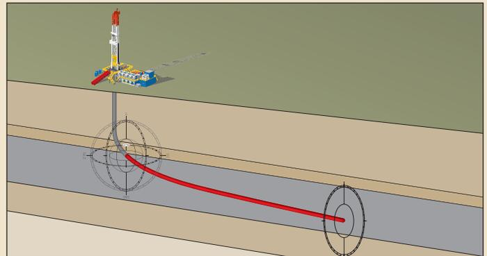
Initially, directional drilling involved a simple rotary bottomhole assembly (BHA) and the manipulation of parameters such as weight on bit (WOB), rotary speed and BHA geometry to achieve a desired trajectory. Changes in BHA stiffness, stabilizer placement and gauge, rotary speed, WOB, hole diameter, hole angle and formation characteristics all affect the directional capability and drilling efficiency of a BHA.
