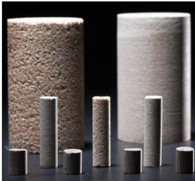
Figure 2. Core samples. If the engineers do not have core samples from the formations, they typically use cores from Berea or Ohio sandstone.
