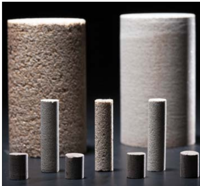
Figure 2. Core samples. If the engineers do not have core samples from the formations, they typically use cores from Berea or Ohio sandstone.
