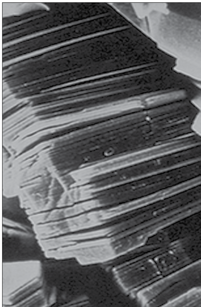
Figure 1. Scanning electron microscope (SEM) photograph of kaolinite clay. The photograph shows the kaolinite aggregates filling a pore. Should these aggregates be allowed to disperse into single particles or platelets, their migration can cause formation damage.
