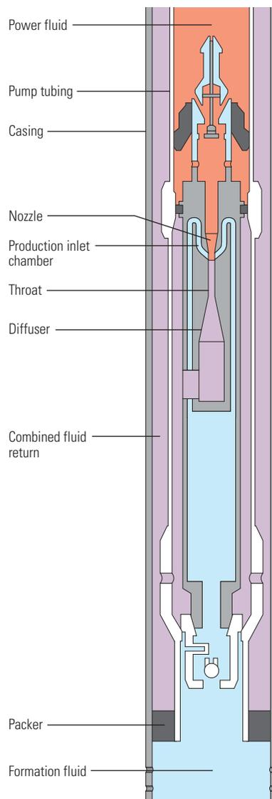
Figure 1. Typical components of a downhole jet pump. Pressurized power fluid from the surface enters the pump from the top and travels through the nozzle. The power fluid mixes in the pump throat with the reservoir fluid, which enters the jet pump from below. The fluid mixture passes through the diffuser, where it picks up sufficient velocity to travel to the surface through the combined fluid return.
