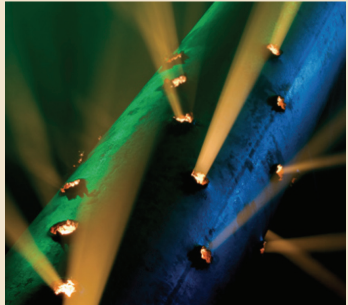
^ High shot density casing gun after perforating.
