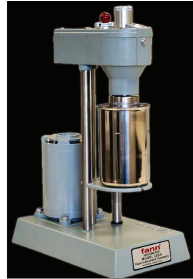
Figure 3. Rheometer. This rheometer is a coaxial cylinder, or Couette, rotational-type viscometer. It consists of an outer cylinder that rotates about an inner cylinder, or bob. Analysts place the test fluid in the gap between the cylinders. The outer cylinder rotates at known velocities. As it rotates, the fluid creates torque, in the form of shear stress, on the inner cylinder. The torque registers as deflections on a precision spring attached to the bob. The spring deflections are observed as direct readings off the display on top of the viscosimeter. Readings are commonly made at 600, 300, 200, 100, 6 and 3 rpm. The readings can be plotted on a chart of shear stress versus shear rate to determine the viscosity and appropriate viscosity model.
