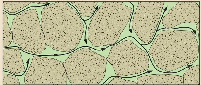
^ The importance of connectivity. Connected pores (green) give rock its permeability, allowing fluid to flow (black arrows).
