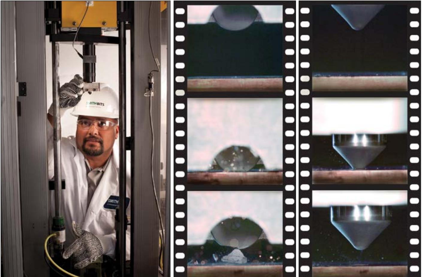
Figure 4. Impact testing. A technician prepares cutters for testing (*left*). Still images from a motion picture indicate that the conventional PDC cutter (*center*, gray rounded element) failed on the first impact; the conical diamond element survived 100 impacts without damage (*right*).
