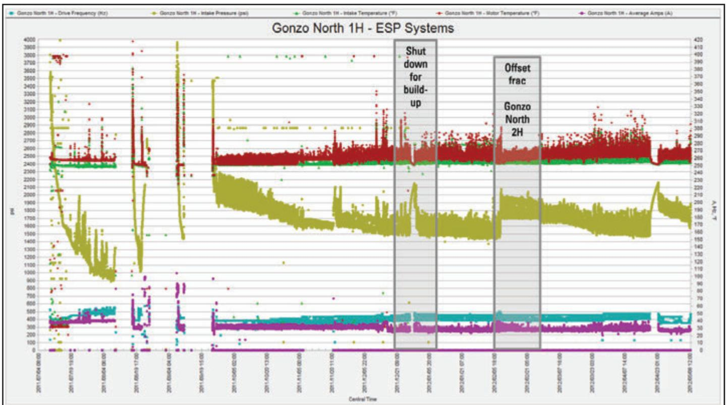
MHR reservoir engineering’s analysis of flowing pressure and corresponding production data using real-time data has been instrumental in the continuous improvement of their artificial lift systems.
