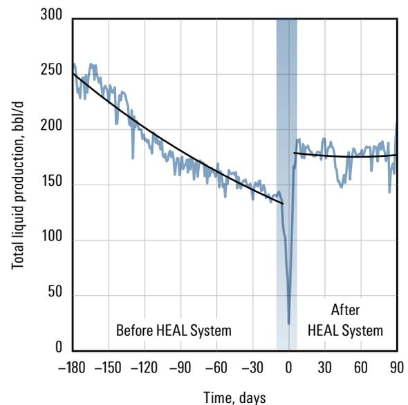
*Total liquid production rate from the seven wells increased significantly compared with using gas lift.*
