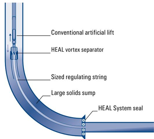
*The HEAL System enhanced rod pumping efficiency by minimizing gas slugs while increasing drawdown.*
