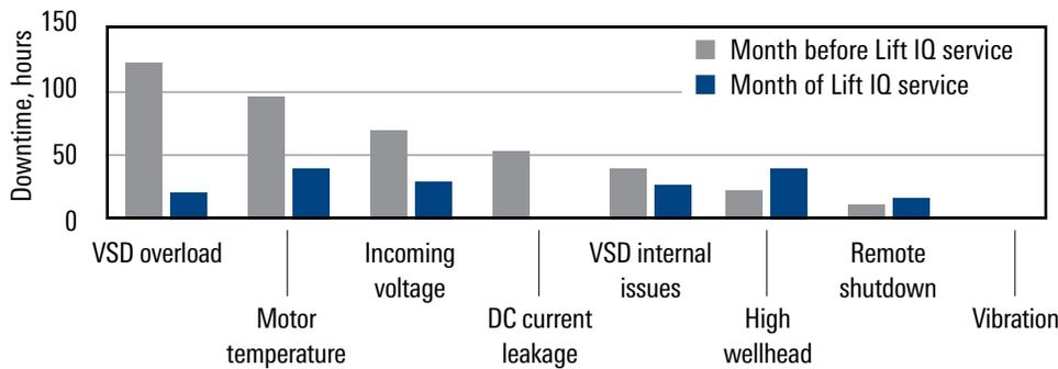
The Lift IQ service reduced the number of ESP shutdowns by 28% and downtime by 56% in two Permian basin fields.
