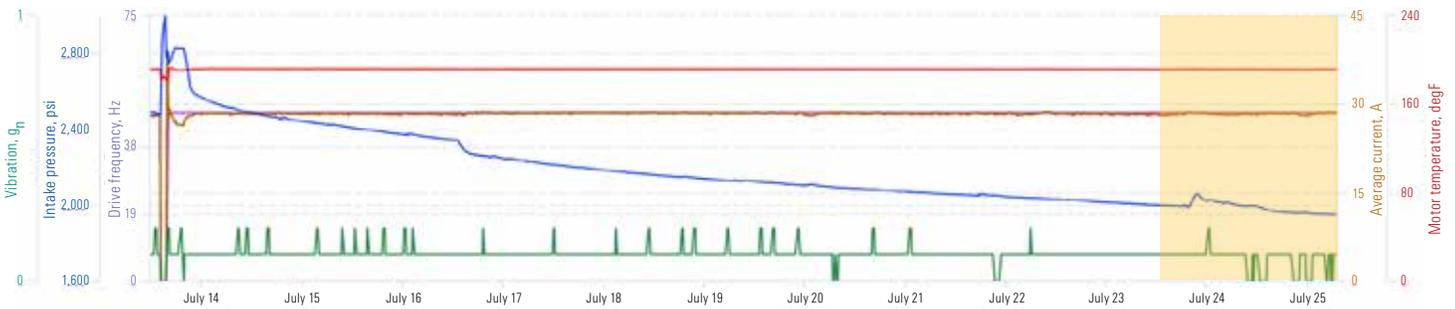
*In one of the five test wells, the ESP intake pressure signature (blue) rises suddenly when the MeshRite screen is plugged and the PumpGuard assembly opens. This pressure signature enables further improvements in production efficiency by predicting the impending sand-related ESP failure so replacement operations can be scheduled.*
