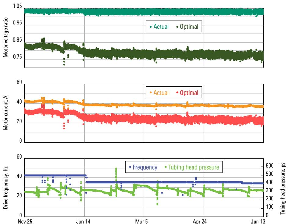
PCL service showed that a 25% reduction in motor voltage on Well B would reduce the current by 14 A—from 38 A to 24 A—without affecting production. Real-time trend analysis provides greater confidence when identifying power optimization opportunities compared with manual single-point analysis. Automated analysis also saves time, an important consideration in fields with large ESP populations.
