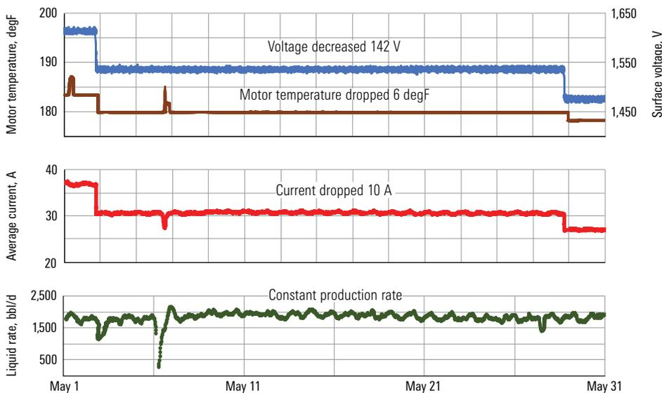
Reduction in wellhead voltage, motor temperature, and current for Well B was achieved via ESP optimization without any loss of production. The voltage reduction was implemented in two steps—on May 3 and May 28—to manage operational uncertainties. This is enabled by Lift IQ service, which allows the surveillance engineer to make changes remotely using two-way SCADA.
