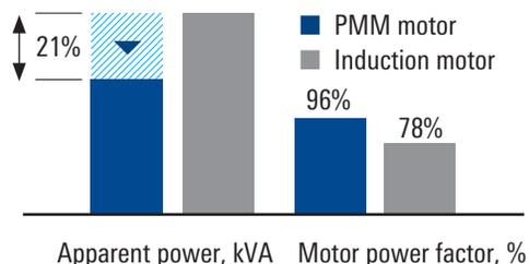
*By installing a permanent magnet motor instead of a conventional AC induction motor to operate an ESP, Cepsa Colombia reduced surface power requirements by at least 21%.*
