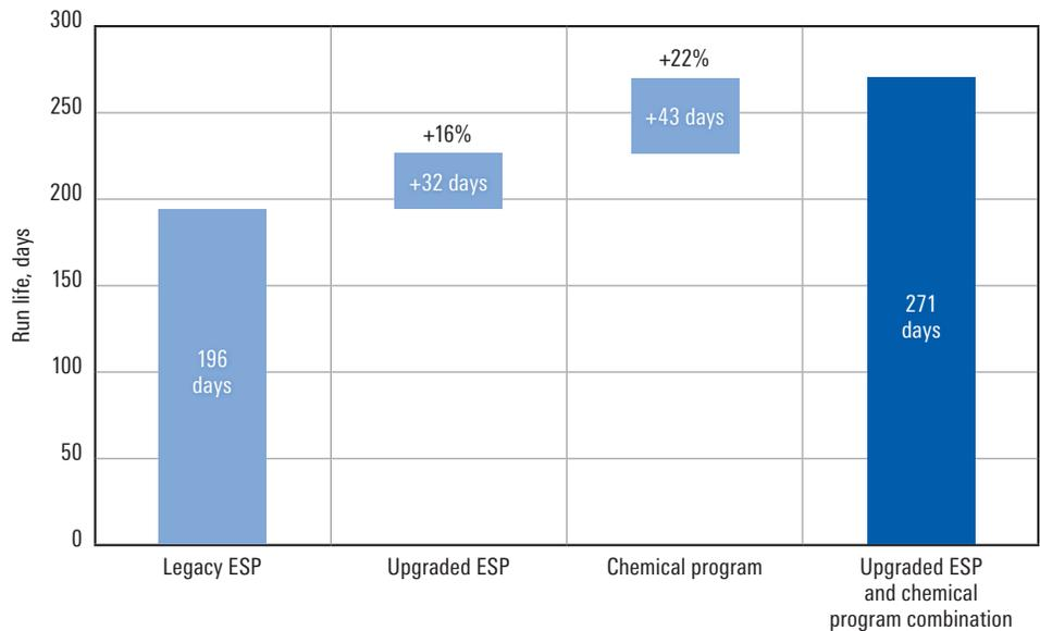
Upgrading ESP components increased run life by 16%, while a custom chemical treatment plan extended it by a further 22% to an average of 271 days.
